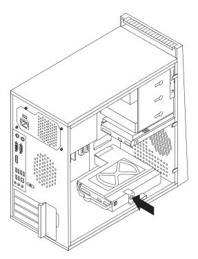
Figure 24. Removing the secondary hard disk drive
